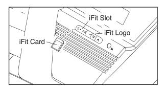
Next, select an iFit workout by pressing the iFit increase and decrease buttons next to the iFit slot. When an iFit workout is selected, the maximum speed setting and the maximum incline setting of the workout will flash in the lower display for a few seconds. In addition, the duration of the workout will appear in the display and a profile of the speed settings of the workout will scroll across the upper display.
